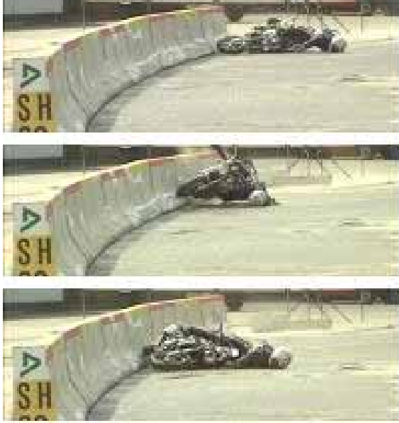
Figure 12. Full-scale crash test where the motorcycle impacts the concrete barrier protection system in a sliding position
