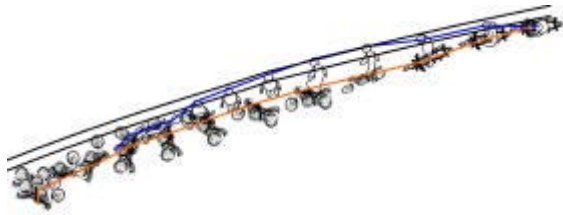
Figure 7. Trajectory of the motorcycle and rider during the first 300 milliseconds after impacting the steel guard rail system EDSP (see Figure 6) determined from analysis of the overhead-view cameras
