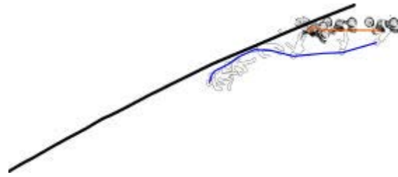
Figure 18. Trajectories of the sliding motorcycle and dummy determined from the overhead view camera before and after impacting into the modified steel guard rail system (see Figure 17)
