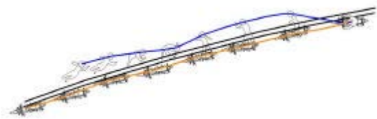
Figure 9. Motorcycle and rider trajectories during the first 175 milliseconds after impacting the concrete barrier (Figure 8) as determined from analysis of the overhead-view cameras
