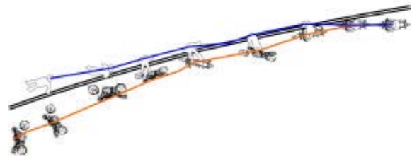
Figure 16. Trajectories of the motorcycle and dummy determined from the overhead view camera before and 230 milliseconds after impacting the modified steel guard rail system (see Figure 15)
